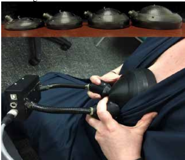
Figure 1. OBS cups and device. Photo demonstrating the four OBS cup sizes in the top photo and the OBS device in use on a participant in the bottom photo
